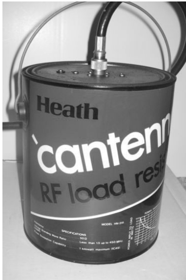
Cantenna dummy load suitable up to 30 MHz and up to 1 kW
