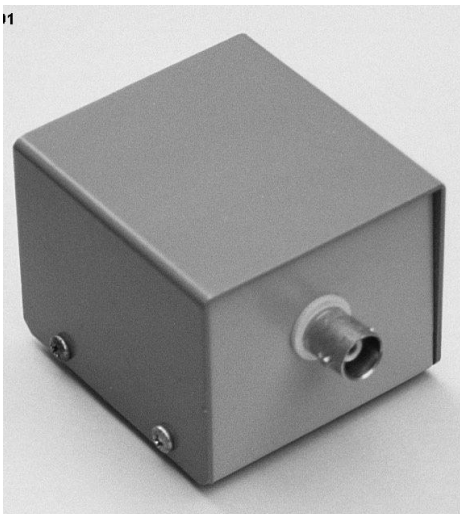
Cantenna dummy load suitable up to 30 MHz and up to 1 kW
